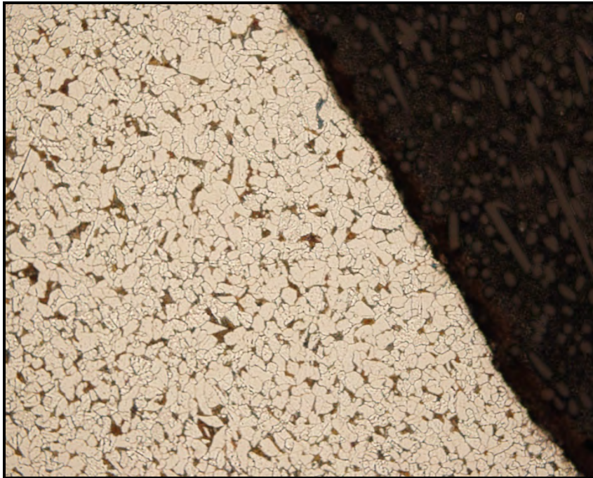
Figure 105: Mount at 7 o'clock: the view shows no corrosion attack on the ID.
