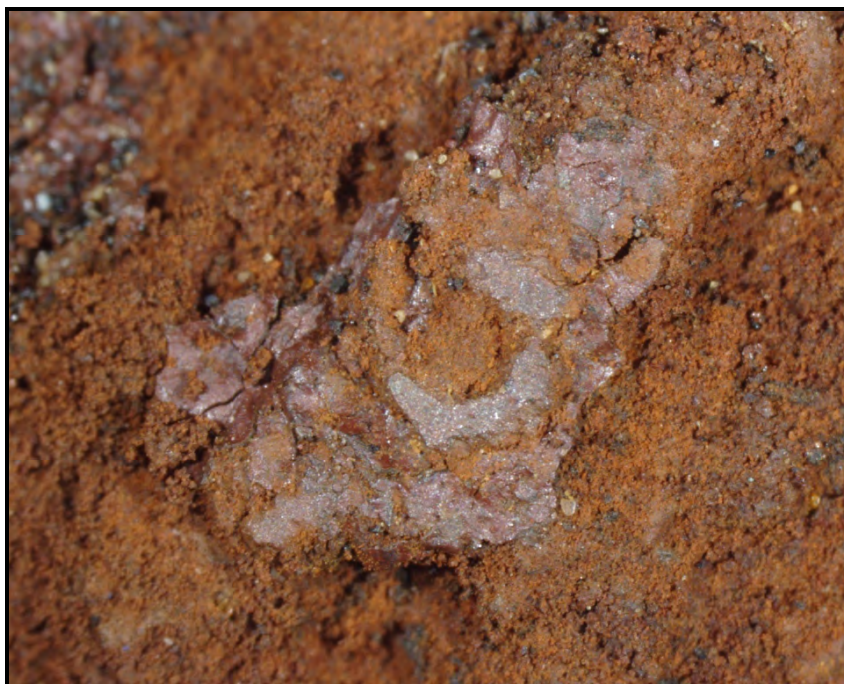
Figure 66: Failed location at 4 o'clock: An overall view of the corroded spot on ID. Note the packed corrosion debris. A higher magnification view of the previous image.
