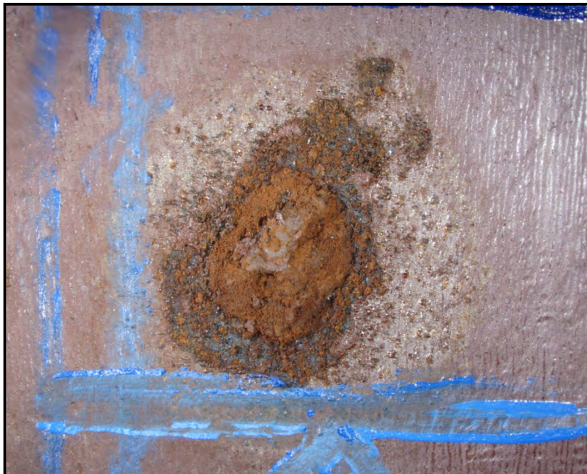
Figure 65: Failed location at 4 o'clock: An overall view of the corroded spot on ID. Note the packed corrosion debris.
